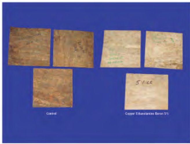
Samples after exposure showing fungal attack (a. Control samples, b. CEB 5%)
