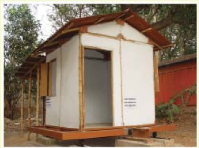
Bamboo House mounted on Shock Table
