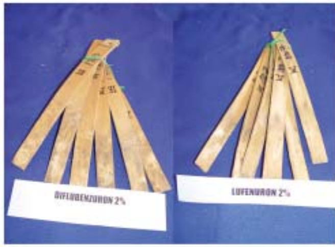
Solid wood samples after Twelve months exposure studies at graveyard
