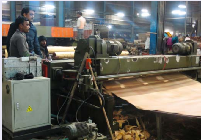
Demonstration on peeling of plantation timber ( Eucalyptus) from spindleless lathe by Shri Uday D.N., Scientist at M/s Green Ply Industries Ltd. Uttarakhand
