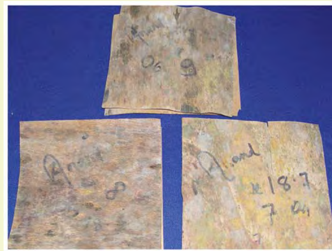
Rubber wood veneer Control samples showing mould attack
